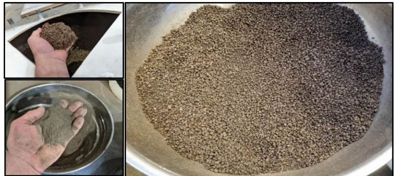
Figure 1. images demonstrate milled manure frass being sieved (<500um) to enable the production of small, regular, granules.
